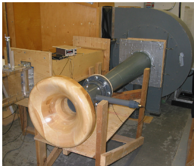
Fig. 3. Experimental set-up showing the inlet contraction and test-section.
